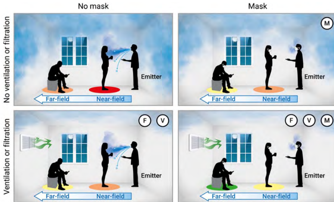
Figure 2: Transmission Paths with and without masks (M) and with and without either ventilation (V) or local filtration (F), from Pohlker et al, https://arxiv.org/abs/2103.01188 . (Note that the image was modified to show ventilation and filtration as graphically represented in the images as a wall-mounted supply air grille, with a window if needed, respectively, for simplicity. Mechanical ventilation from HVAC systems is the primary form of ventilation at 4CD buildings.)
